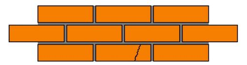
Identify the damaged brick slip and assess whether the brick slip is sufficiently damaged to require replacement.
