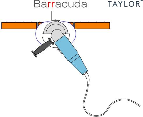
Using the 150mm diameter diamond cutting disc, cut all the way through the damaged brick slip, and the two brick slips immediately above. Ensure that the cut depths are no greater than 42mm and that the cuts do not extend into the adjacent brickwork. A small 'quadrant' of each brick slip will remain un-cut, which will need to be broken. Be careful not to cut into the Barracuda rail, its fastenings or sub-structure.
