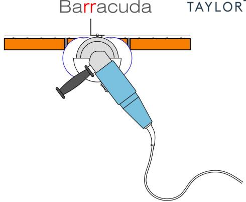
Using the 150mm diameter diamond cutting disc, cut all the way through the damaged brick slip, ensuring that the cut depth is no greater than 42mm and that the cuts do not extend into the adjacent brickwork. A small 'quadrant' of brick slip will remain un-cut, which will need to be broken. Be careful not to cut into the Barracuda rail, its fastenings or substructure.
