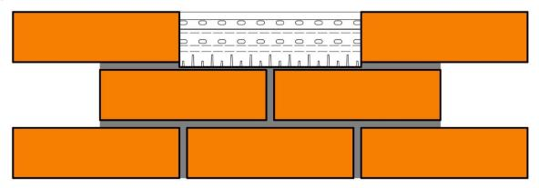
Remove the mortar from the vertical joints. The finished, prepared surfaces, should look like this.
