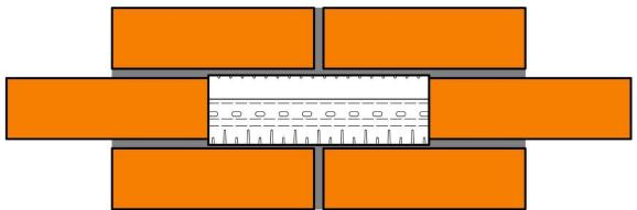
Remove the mortar from the vertical joints. The finished, prepared surfaces, should look like this.
