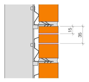
If the brick slip does require replacement, carefully mark two horizontal cut positions onto the face of the damaged brick slip. The centre of one cut must be 15mm below the top of the damaged brick slip and the centre of the other, 35mm below the top of the damaged brick slip.
