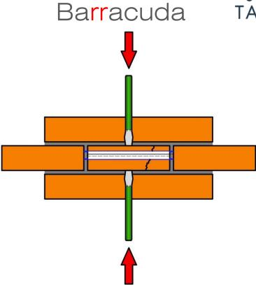
Using the small sharp cold chisel, carefully break out the top and bottom portions of the damaged brick slip.
