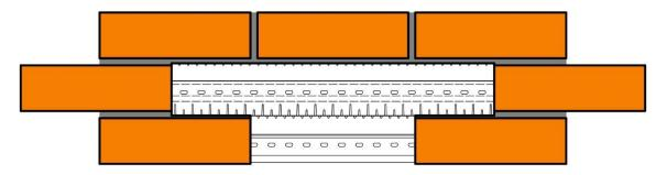
Remove the mortar from the vertical joints. The finished, prepared surfaces, should look like this.
