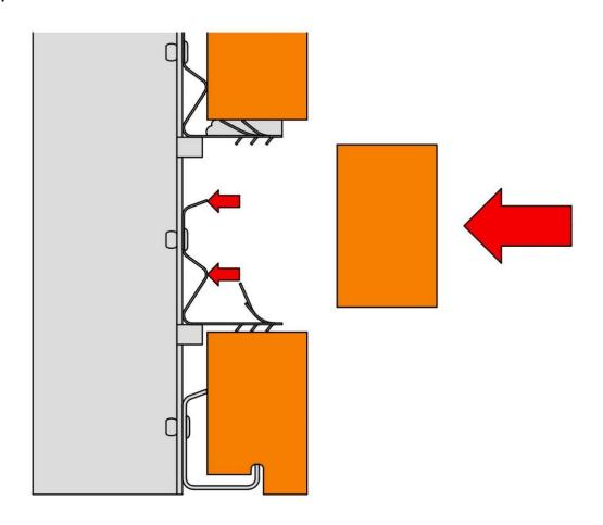
Push the replacement brick slips into place in the course immediately above the replacement brick location. Use the blond dead blow mallet if necessary.
