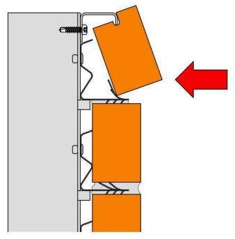
Blow or vacuum any brick and mortar dust from the surfaces of the Barracuda rails and the adjacent brickwork and push the replacement brick slip into position. Use the blond dead blow mallet if necessary.
