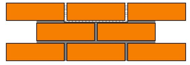
Make sure that the replacement brick slip is fully inserted and secure, and that the width of the vertical joints each side of the replacement brick slip are approximately equal.
