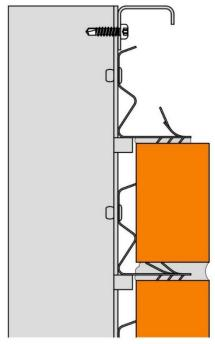
Carefully remove the mortar that encapsulates the horizontal rail teeth and dress the mortar back to the leading edge of the horizontal rails as shown. The teeth are extremely durable and can be bent upwards so that they effectively capture the replacement brick slip.
