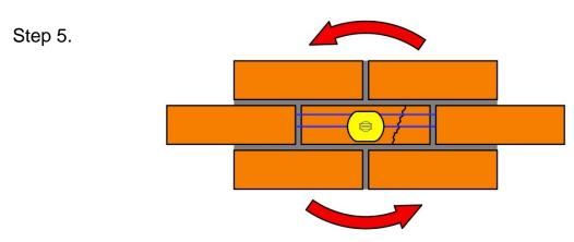
Insert the large 'flat blade screw driver into the middle of each cut. Twist the screw driver to fracture the middle portion of the damaged brick slip.
