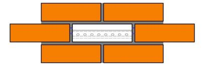
Start to carefully remove the mortar that surrounded the damaged brick slip.
