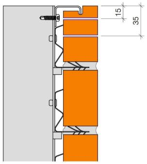
If the brick slip does require replacement, carefully mark two horizontal cut positions onto the face of the damaged brick slip. The centre of one cut must be 15mm below the top of the damaged brick slip and the centre of the other, 35mm below the top of the damaged brick slip.
