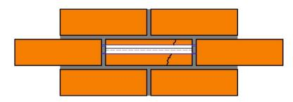
Remove the middle portion of the damaged brick slip.
