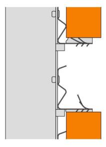
Carefully remove the mortar that encapsulates the horizontal rail teeth and dress the mortar back to the leading edge of the horizontal rails as shown. The teeth are extremely durable and can be bent upwards so that they effectively capture the replacement brick slip.
