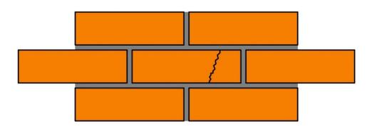
Identify the damaged brick slip and assess whether the brick slip is sufficiently damaged to require replacement.
