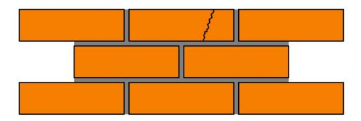
Identify the damaged brick slip and assess whether the brick slip is sufficiently damaged to require replacement.
