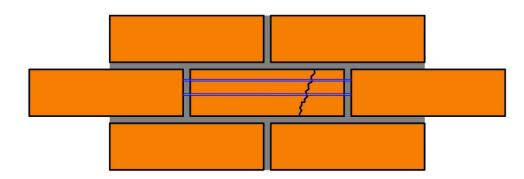
Using the 150mm diamond cutting disc, start to make two [initially shallow] cuts for the full length of the damaged brick slip, extending into the perpend joints between the damaged brick slip and the adjacent brickwork. Be careful not to cut into the adjacent brickwork.
