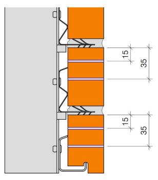
If the brick slip does require replacement, carefully mark two horizontal cut positions onto the face of the damaged brick slip and the two brick slips immediately above the damaged brick slip. The centre of one cut must be 15mm below the top of each brick slip and the centre of the other, 35mm below the top of each brick slip.
