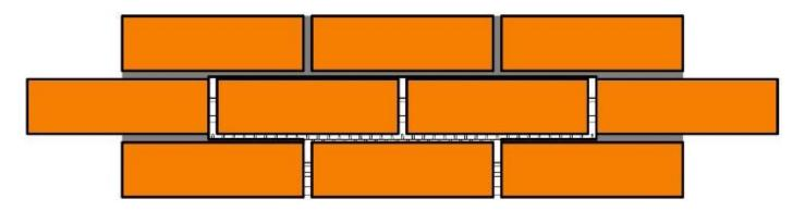
Make sure that all replacement brick slips are fully inserted and secure and that the width of the vertical joints each side of the replacement bricks are approximately equal.
