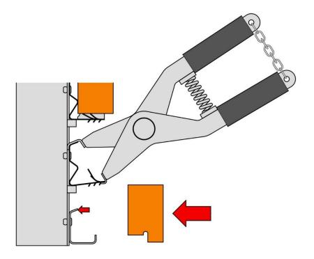
Blow or vacuum any brick and mortar dust from the surfaces of the Barracuda rails and the adjacent brickwork. Use the Bottom Brick slip Installation Tool to compress the rail above the centre of the damaged brick slip location and push the replacement brick slip into position. Use the blond dead blow mallet if necessary.
