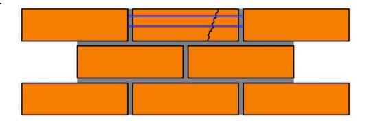
Using the 150mm diamond cutting disc, start to make two [initially shallow] cuts for the full length of the damaged brick slip, extending into the perpend joints between the damaged brick slip and the adjacent brickwork. Be careful not to cut into the adjacent brickwork.
