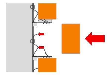
Blow or vacuum any brick and mortar dust from the surfaces of the Barracuda rails and the adjacent brickwork and push the replacement brick slip into position. Use the blond dead blow mallet if necessary.
