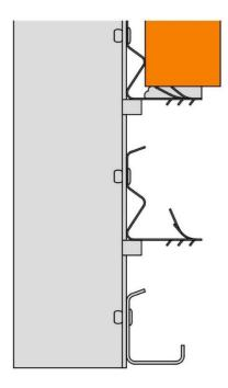
Carefully remove the mortar that encapsulates the horizontal rail teeth and dress the mortar back to the leading edge of the horizontal rails as shown. The teeth are extremely durable and can be bent upwards so that they effectively capture the replacement brick slips.
