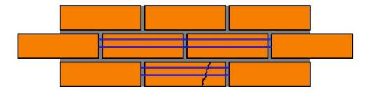
Using the 150mm diamond cutting disc, start to make two [initially shallow] cuts for the full length of the damaged brick slip, and the two brick slips immediately above. Extend these cuts into the perpend joints between the brick slips that require removal and the adjacent brickwork. Be careful not to cut into the adjacent brickwork.
