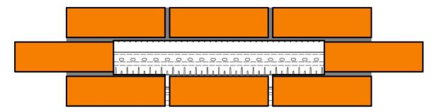
Make sure that the replacement brick slip is fully inserted and secure, and that the width of the vertical joints each side of the replacement brick slip are approximately equal.
